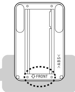
Set up the drive and stand so that "FRONT" on the underside of the stand faces forward (towards the disk slot).
