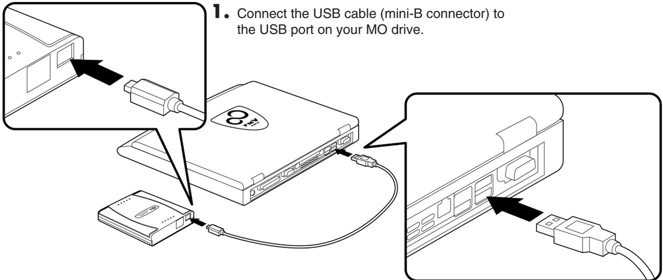
**1.** Connect the USB cable (mini-B connector) to the USB port on your MO drive.
