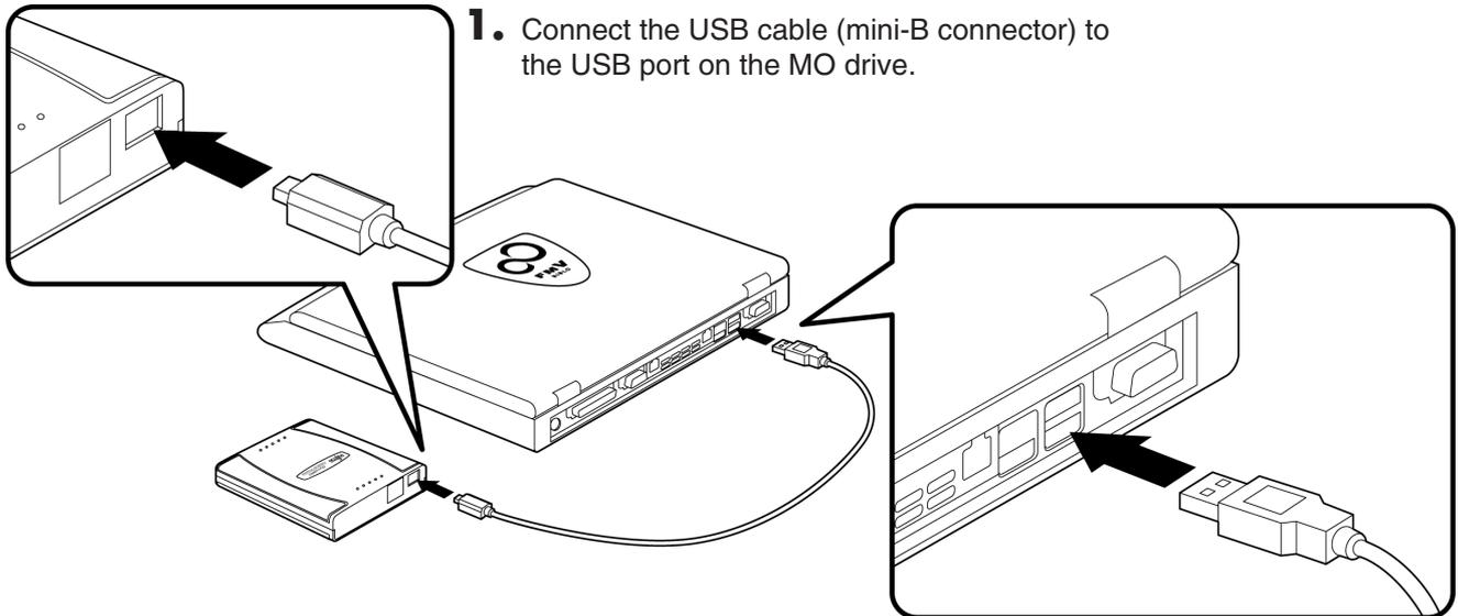
**1.** Connect the USB cable (mini-B connector) to the USB port on the MO drive.
