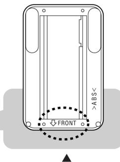
Set up the drive and stand so that "FRONT" on the underside of the stand faces forward (towards the disk slot).
