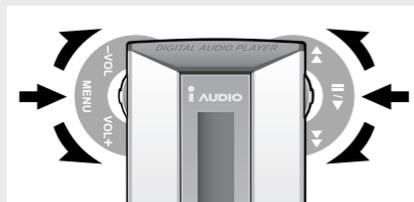
For PLAY/STOP, and MENU, press the jog lever inward, and for REW, FF, + VOL, and VOL -, push the jog lever up or down.
