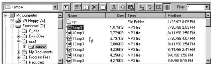
JetShell's file management window looks very similar to Windows Explorer. In the left window, hard drives and CD-ROM drives attached to PC and the folders contained in them are displayed. In the right window, the files that are contained in the selected folder are displayed.
