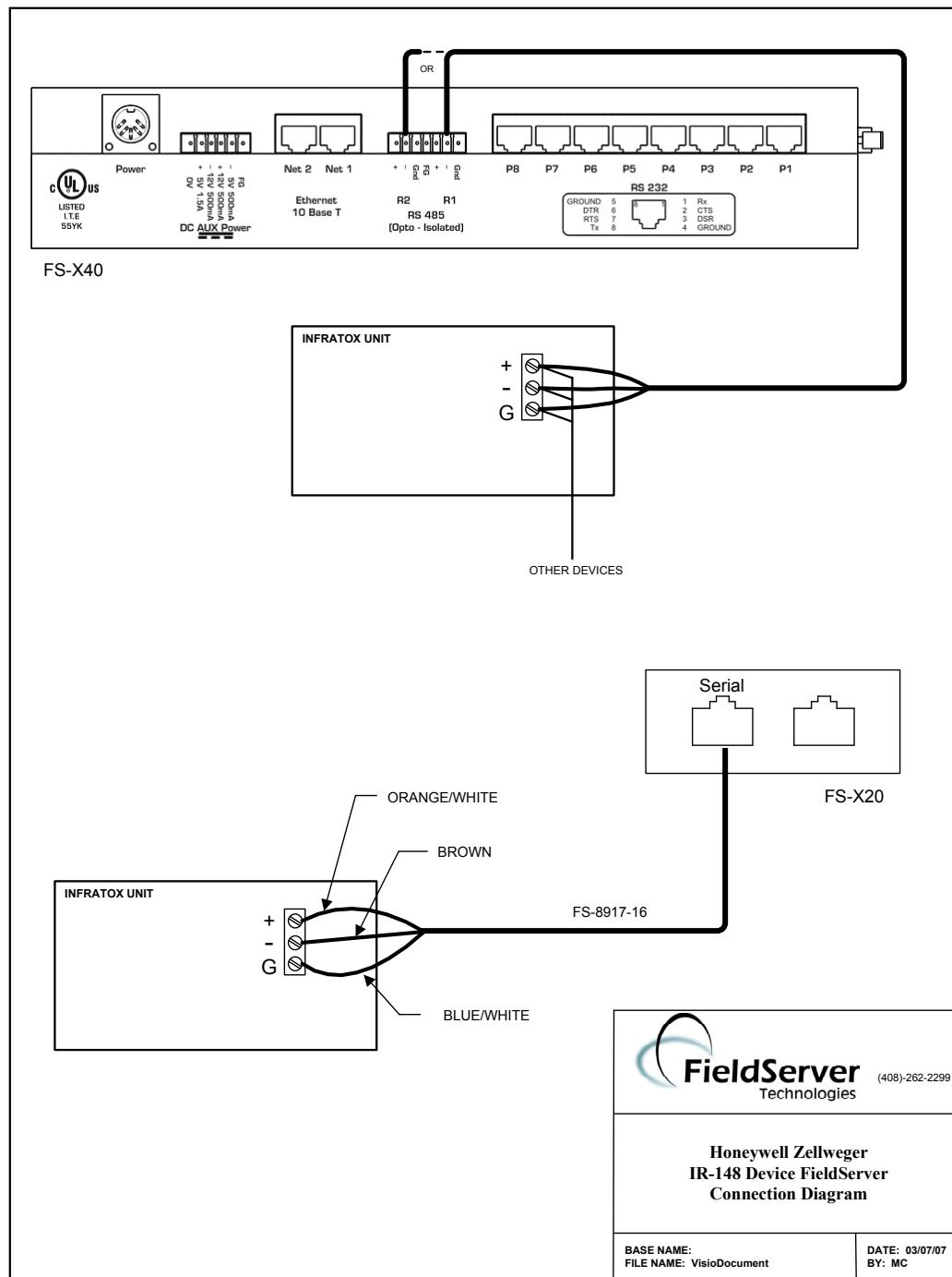
\*Other devices must not transmit Honeywell Zellweger IR-148 49 byte messages
