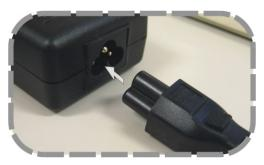
2. Connect the connector end to the device and the plug to an outlet.
