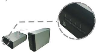
2. Unscrew the screws on both the top and bottom side of the device.
