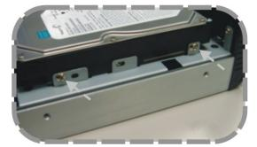
6. Place the HD cover back on to the device and screw the cover on.
