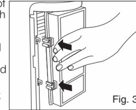
8. Replace air inlet grill back onto unit securely.
