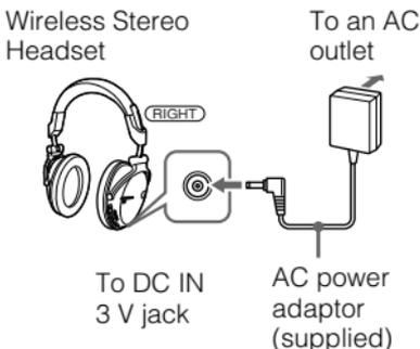
When the AC power adaptor is connected to an AC outlet, charging starts.
