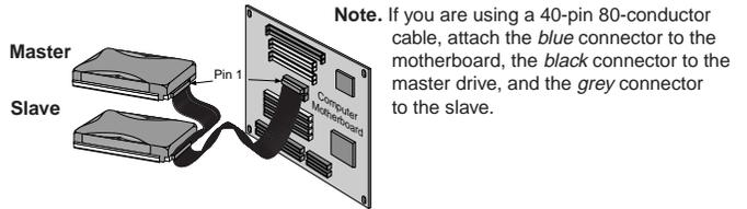
2. Attach the interface connector and the power connector to the drive.
