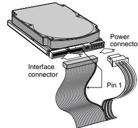
**Note.** You can mount the drive in any orientation. Usually it is mounted with the circuit board down.
