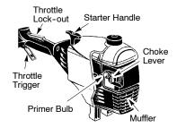
**NOTE:** The throttle lock-out must be engaged to allow operation of the throttle trigger. The lock-out is engaged with the palm of your hand as you grip the throttle handle.
