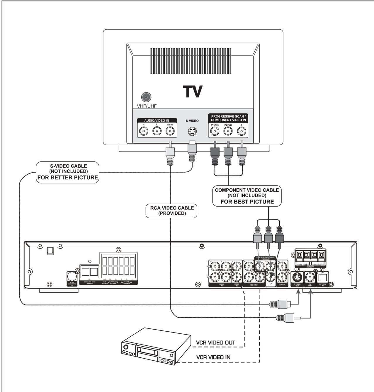
**NOTE:** When in AV1 or AV2 mode, only composite video sources will have video output signal, therefore, connect only RCA video output or TV Out to your TV sets.
