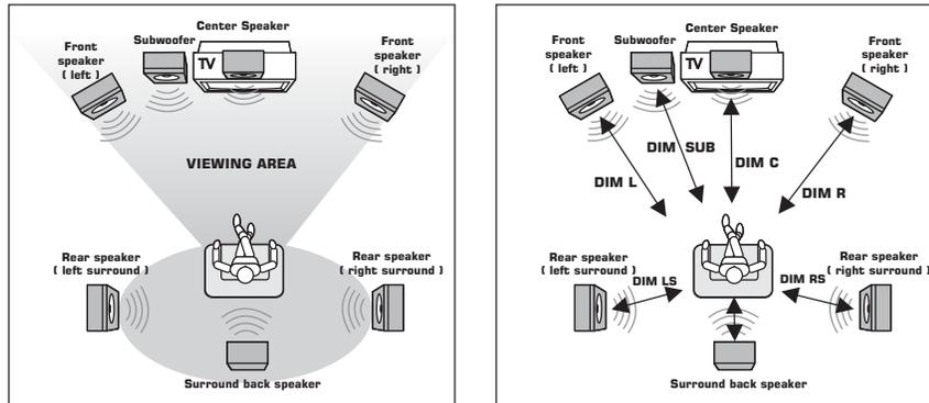
A typical room layout will have the left, center, and right speakers placed across the front and the left surround and right surround speakers placed along the sides towards the rear and the back surround speaker placed right behind the listener as shown in the above left picture. The center speaker can be positioned above or below the video screen or TV. A subwoofer can be installed for powerful bass sounds and can be positioned anywhere in the room.
