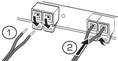
Fully insert the stripped portion of the antenna into the terminal as shown above.
