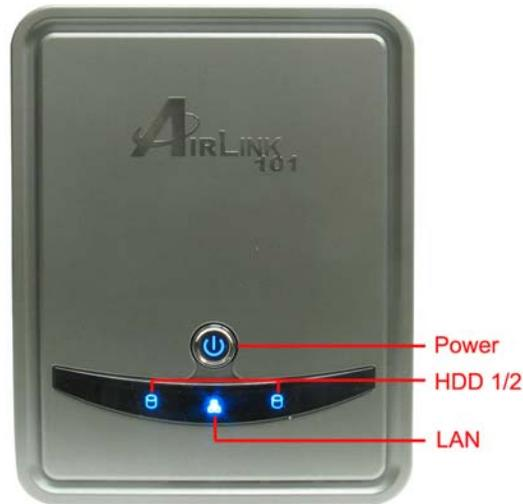
**1. Power LED** – The steady **Blue** light indicates the server is powered on. This LED will be off when the 2-Bay NAS is on power saving mode.
