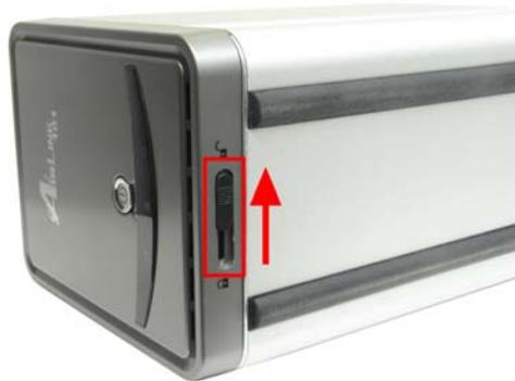
**Step 2** Slide the front panel up and then pull it off to access the drive bays.
