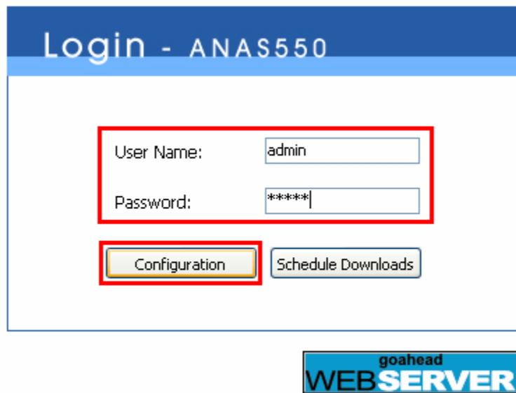
If you ever change the username or password and forget, you will need to perform the factory reset procedure to reset the system to factory defaults. To do this: Press and hold the **Reset** button on the back panel for 10 seconds to reset the device to factory default settings.
