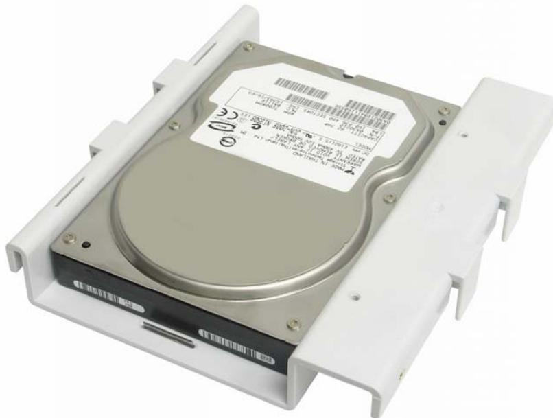
**Step 6** Turn the plate over and secure the hard drive to the plate with the provided four screws.
