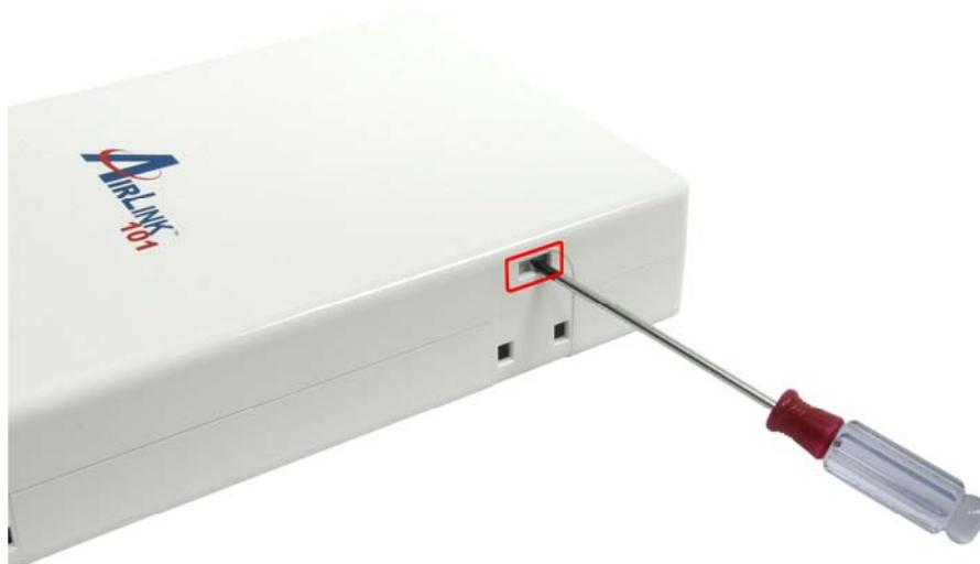
**Step 4** Remove the two screws holding plate A and then remove plate A from plate B.
