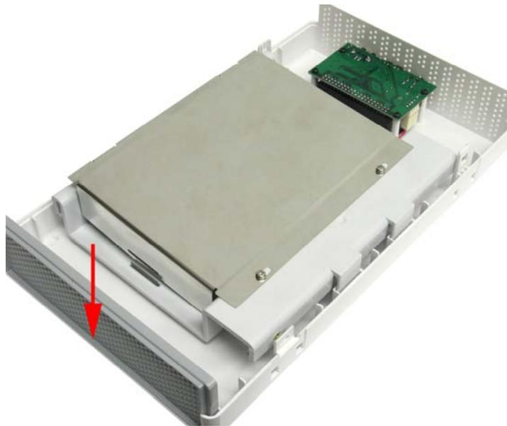
**Step 10** Replace the top cover and re-secure the screws removed in Step 1.
