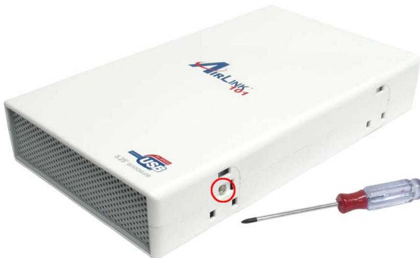
**Step 3** Remove the top cover. If you find it hard to open the cover, use the screwdriver to slightly push the locking tab inside.
