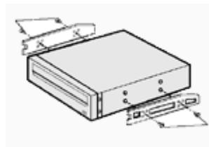
4. Insert the DVD Writer after removing the plate as below.
