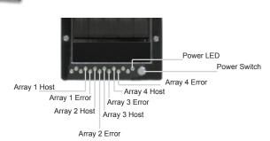
Power LED: lit when RAID Tower is on.
