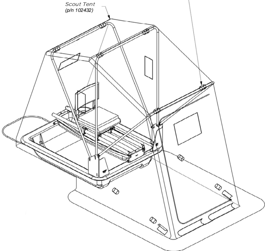
***Remove the Rear Adjustable Spreader Pole after you have fastened the Roof Velcro.***
