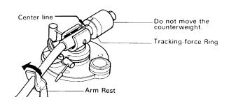
• Pull up the Arm Rest and turn it counterclockwise so that the Arm Rest returns to its original position. Secure the Tonearm to the Arm Rest again.
