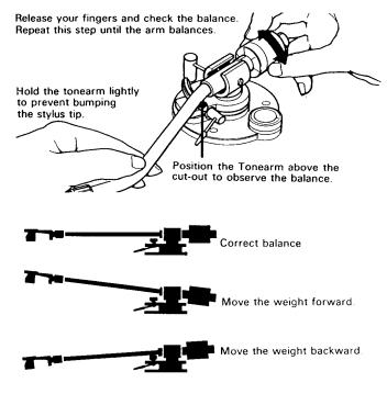
**6** While holding the Counterweight at the balanced position, separately turn the Tracking-force Ring until the "0" indication meets the center line on the Tonearm. Recheck the balance.
