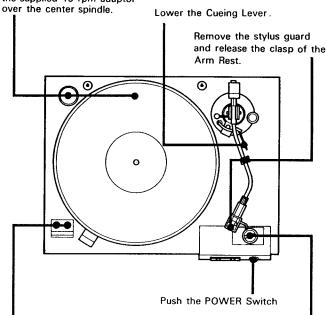
Push either the "33" or "45" -rpm Button according to the record speed.
