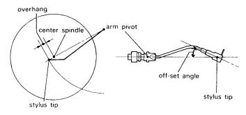
Tracking error is minimized by the selection of an optimum "off-set" angle and "overhang" distance. Overhang is the distance between the stylus tip and the center spindle. This overhang adjustment is made at the time of installing a particular cartridge, while the off-set angle is fixed by the manufacturer of the tongarm.
