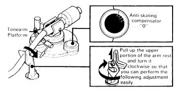
❸ Turn the Counterweight as required until the Tonearm is in a horizontally balanced position. (The Tracking-force Ring turns simultaneously.)
