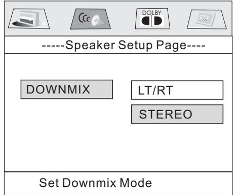
This is to activate the audio output from DOLBY AC3 5.1 DOWNMIX to 2 channel mode. Select the preferred SPEAKER connection by using the cursor buttons. Select the LT/RT to activate the Dolby surround compatible output. Select the STEREO to activate simple stereo mode.
