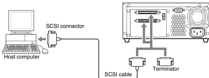
A SCSI bus allows you to connect up to fifteen peripherals to the host computer, including the unit.
