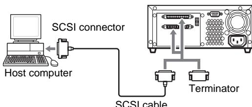
A SCSI bus allows you to connect up to fifteen peripherals to the host computer, including the unit.
