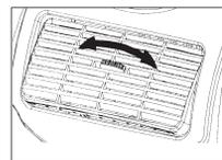
Turn the roller on the air vent to control the airflow direction from the vertical louvers.
