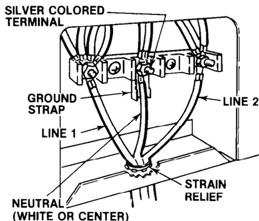
Use this wiring method **ONLY** if local codes permit connecting frame grounding conductor to neutral wire of power cord.
