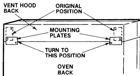
Loosen screws holding the 2 mounting plates on the back of the vent hood. Rotate these plates (as shown) until the lower holes line up with matching screwholes in the back of the oven.
