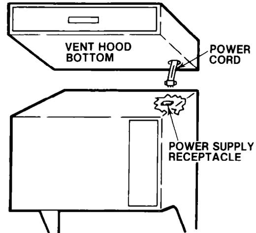
Reach through hole in bottom of vent hood, pull out power cord until all slack is removed.
