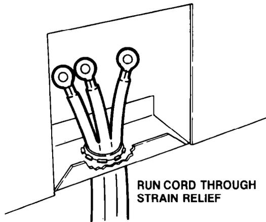
Run cord or cable through strain relief. Leave enough slack to attach ring-type terminals to terminal block. Tighten clamping screws.
