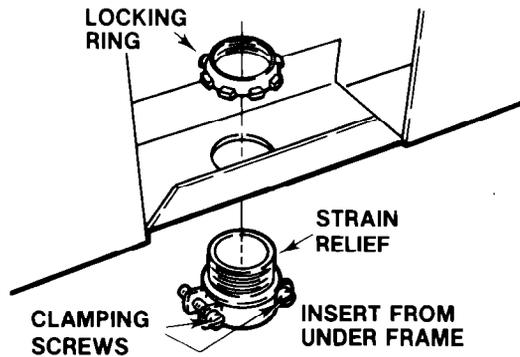
Disconnect clamping ring from strain relief. Push relief (from bottom) through hole beneath terminal block. Tighten clamping ring (from above) onto strain relief threads.
