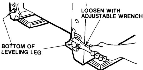
Once skid is removed, 4 leveling legs are exposed at bottom of frame.
