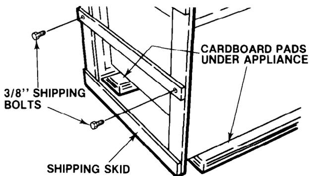
Remove the 4 cardboard pads from shipping box. Place them on floor as shown to protect appliance's finish. Rest appliance (on its back) on pads.
