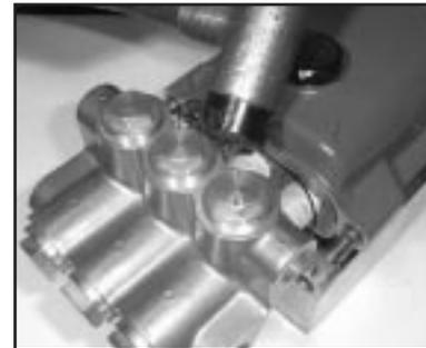
firmly into the retainer with a wooden dowel making certain that the spring side of the seal is installed first and that the seal sits squarely in the retainer.
