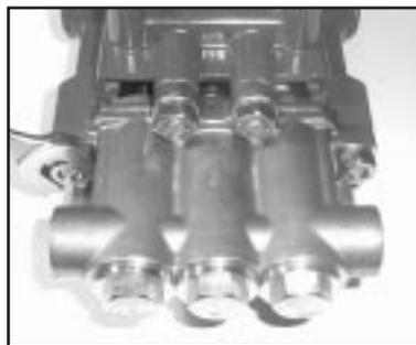
8. Drain the oil from the pump. Turn the pump over to remove the four manifold stud nuts (46) with a 19mm wrench.
