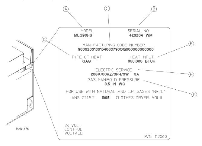
When contacting **ADC**, certain information is required to ensure proper service and parts information. This information is on the data label, located on the top right corner of the dryer, viewed from the rear (refer to illustration). When contacting **ADC**, please have the model number and serial number readily accessible.
