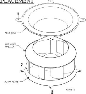
**NOTE:** The motorized impellor assembly <u>will not be</u> able to be removed due to the wiring harness still connected.
