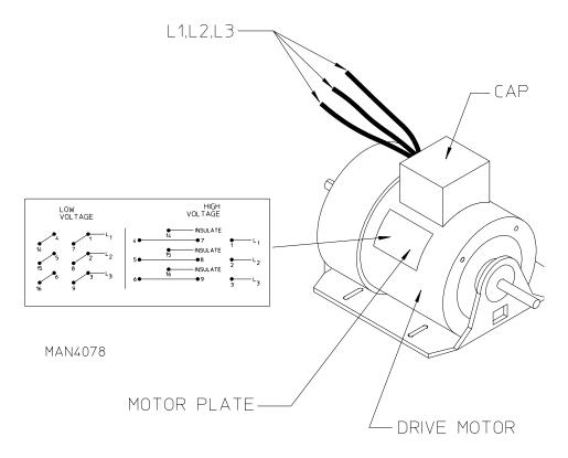
The motor plate is located on the side of the drive motor (refer to illustration) and contains a graphical representation of the motor wiring for both low and high voltage ratings.
