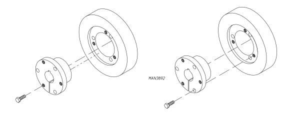
**IMPORTANT:** Tighten screws evenly and progressively. Never allow the sheave to be drawn in contact with the flange of the bushing. This gap should measure from 1/8" to 1/4". Proper cap screw torque is 30 ft-lbs. (41 Nm). If greater tightening forces are applied, excess pressure will be created in the hub of the mounted sheave which may cause it to crack.
