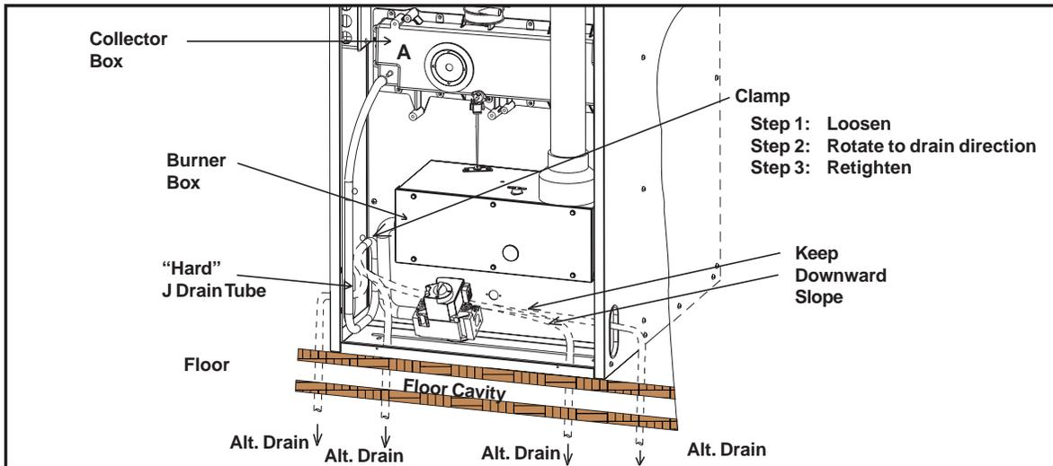
**Figure 21. Furnace with Condensate Drain Trap Assembly**
