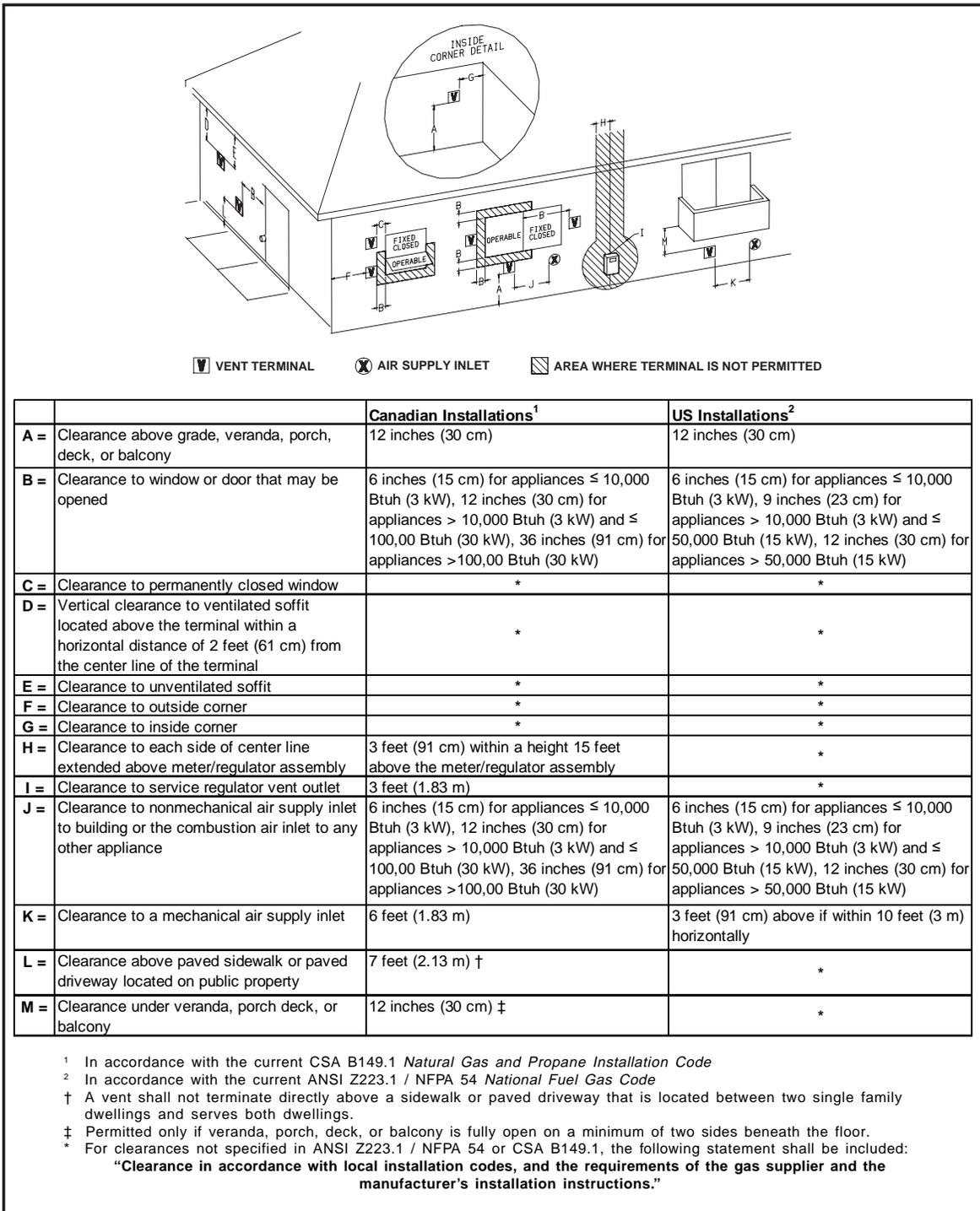
Figure 15. Vent Termination Clearances for Direct Vent Furnaces
