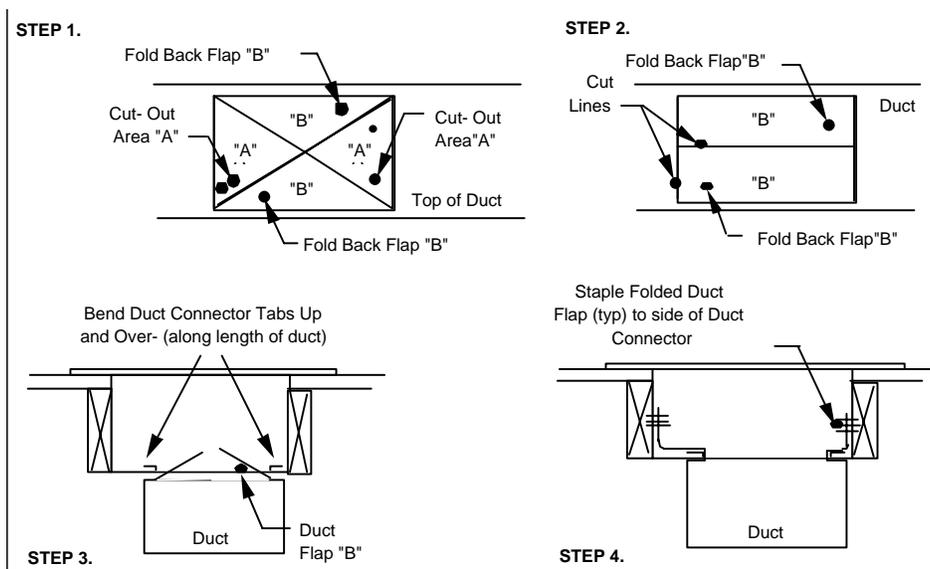
Figure 12. Alternate Installation
