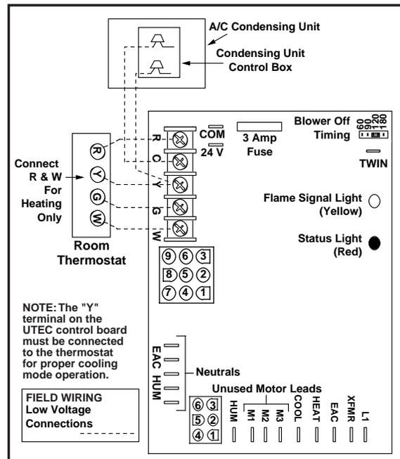
**Figure 28. Low Voltage Field, Four-wire Heating/Cooling Applications**
