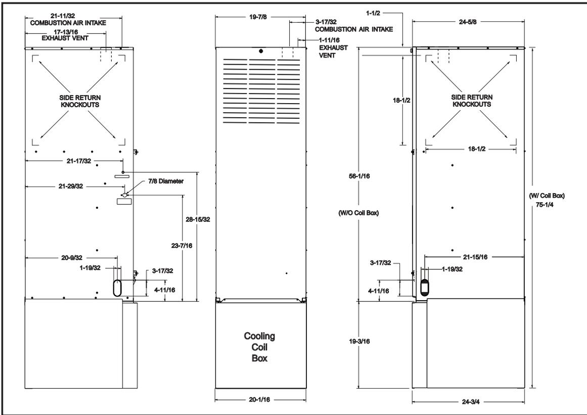
Figure 1. Furnace Dimensions
