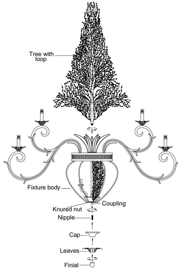
1. Before beginning the assembly, carefully unpack and identify all parts referring to the illustration.
