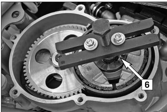
Screw the extractor (special tool item no. 590.29.021.044) onto the clutch hub [6] with the M5x50 screws, hold the extractor and remove the centrifugal clutch from the crankshaft by screwing in the extractor screw. Completely remove the centrifugal clutch, bearings and spacing washers from the crankshaft.
