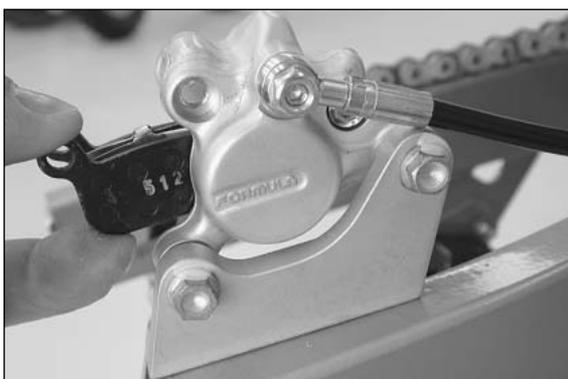
Slide new brake shoes into the brake caliper a fasten with the screw [5].
