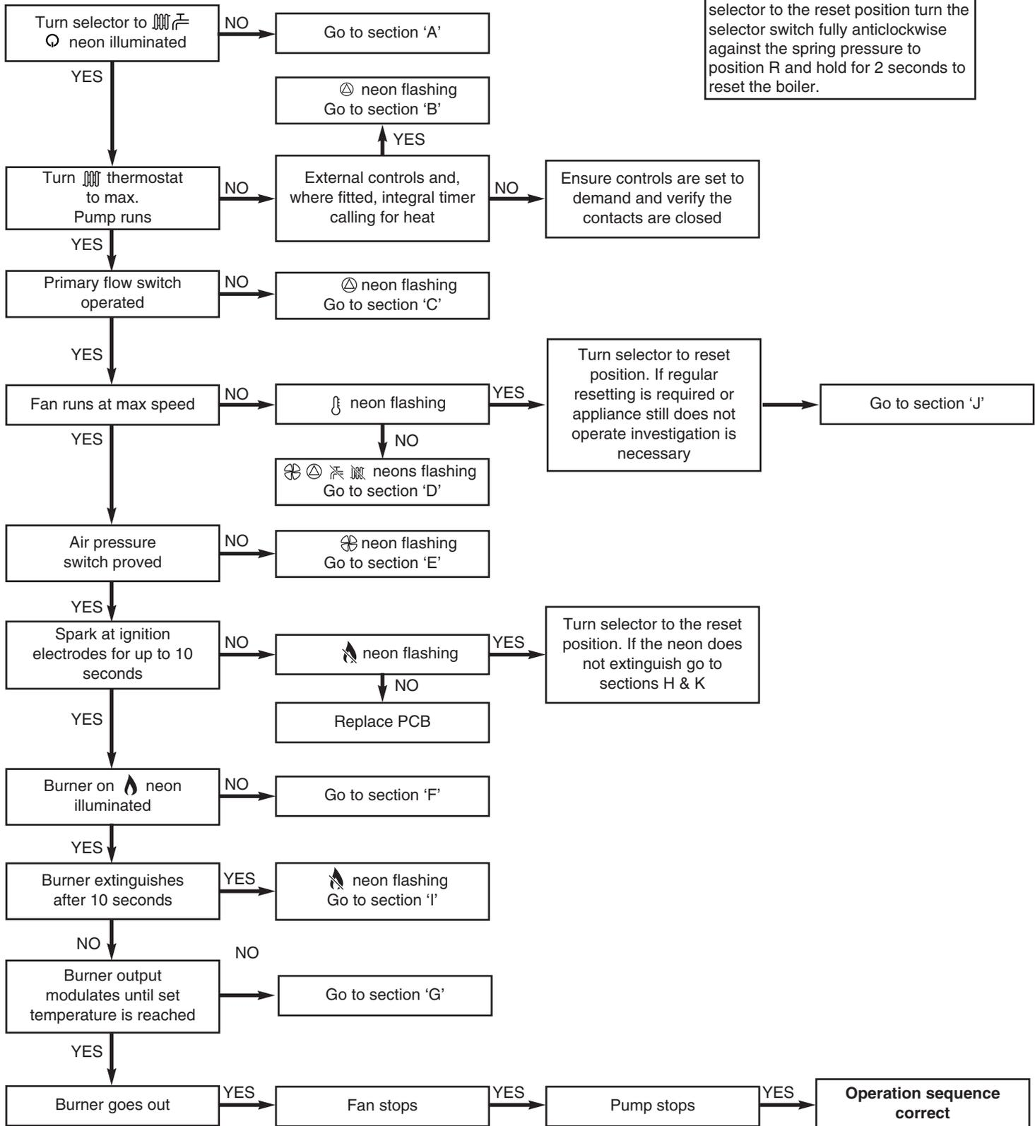
**NOTE:** When instructed to turn the selector to the reset position turn the selector switch fully anticlockwise against the spring pressure to position R and hold for 2 seconds to reset the boiler.
