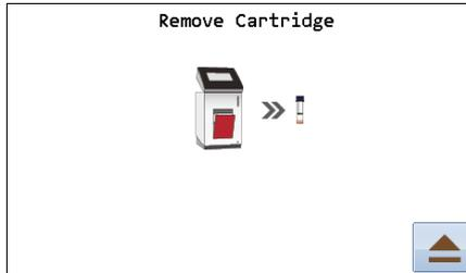
The instrument automatically opens the door. Remove the test cartridge and discard it. Touch to close the door. The main menu appears.
