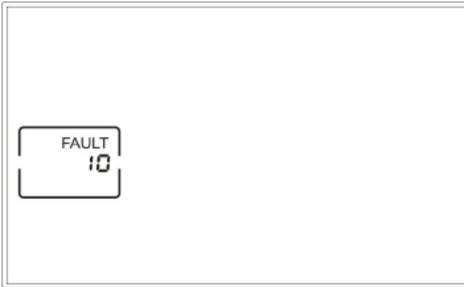
Communication Fault mode
