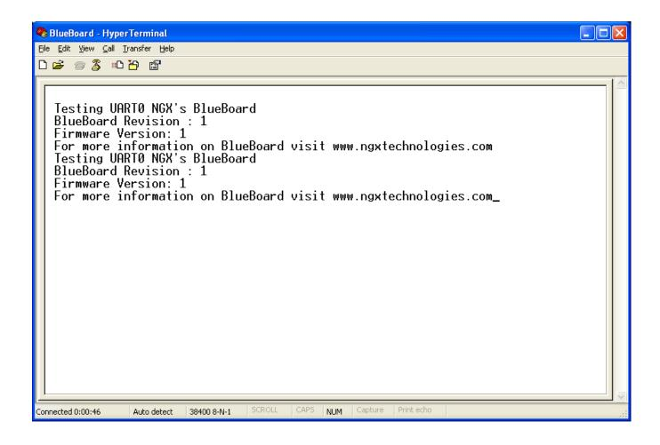
UART0 can also be used for serial programming. If the selected bootloader mode is Manual then Half modem cable should be used, else if it is in Auto mode use full modem cable. Note that after programming in auto mode the serial cable should be disconnected.
