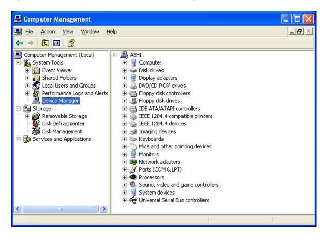
The device uses the *usbser.sys* driver. This driver file is not unpacked in Windows by default and needs to be extracted from a Windows .cab file which should be in the C:\WINDOWS\Driver Cache\i386 directory for Windows XP SP2. Change directory to **C:\WINDOWS\Driver Cache\i386** expand the CAB file by running the below command in Command-Prompt
