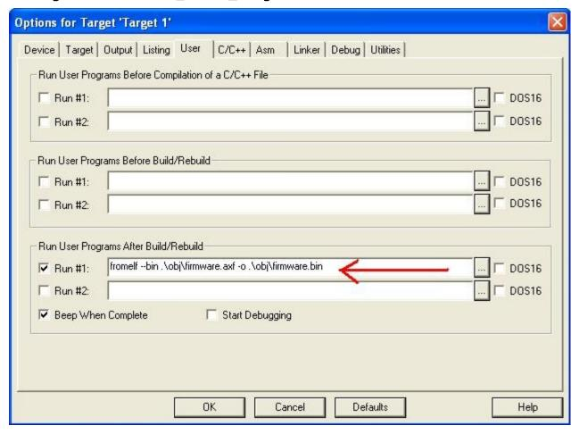
Insert the user command in Run #1 ticking the check box. After compile and build the entire project, from elf it creates hex file along with the hex file there will be another file with the extension .axf. This user command is used to convert .axf file to .bin. Here in fig. Above firmware.axf is converted to firmware.bin which is used for drag drop programming with the USB boot-loader that allows you to enumerate the board as a Mass Storage Device.
