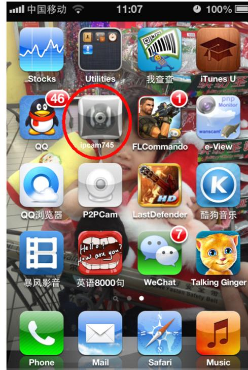
3.Run the app "ipcam745", press "New"and "Refresh" to find the camera's ip address in the Lan,select an ip you need to view.
