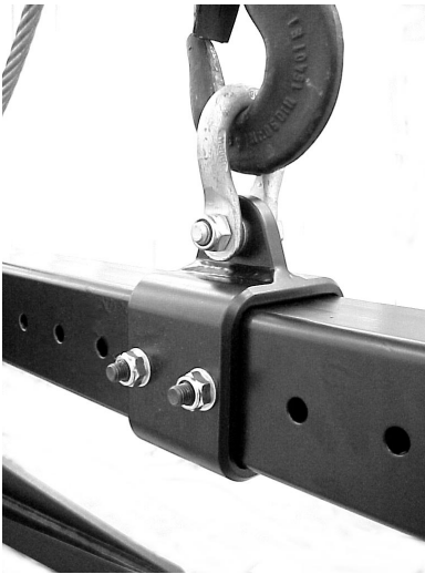
Lifting slider mounted on the box section
