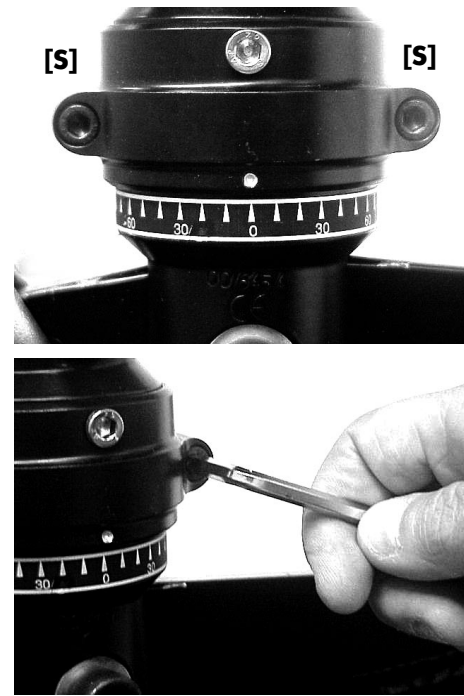
Tightening the clamping screws [S] on the rota swivel
