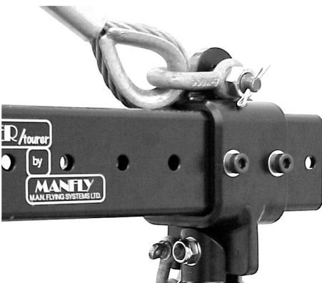
A safety wire fastened correctly in a suspension eye
