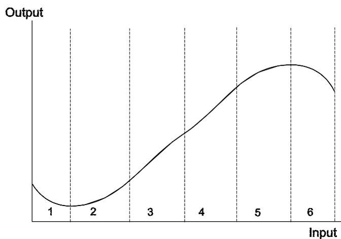
PReset must calculate 4 coefficients  $a_0$ ,  $a_1$ ,  $a_2$  and  $a_3$  for all 6 sections including 5 section limits, indicating curve sections for 0 -100% of the input span. This means that PReset must transfer all together 5 section limits and 24 coefficients to PReTrans or PReview. These calculations are rather cumbersome, thus PReset offers three alternative ways to enter data:
