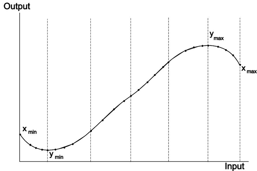
**Note:** Highest and lowest input values (Xmax and Xmin) plus highest and lowest output values (Ymax and Ymin) must be among the entered values as linearisation is scaled according to these values.
