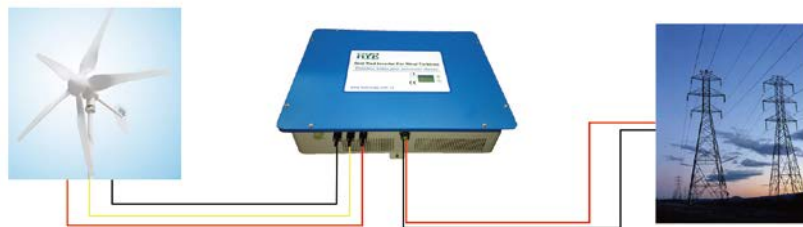
Fig. 1: Principle block diagram of HYGCI-15CL (V1.0/V1.5) between small wind turbine and grid
