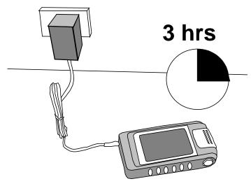
The red light beside the power connector should illuminate indicating that the battery is being charged. The light will go off when the battery is substantially charged. It takes about three hours to charge the battery from a discharged state. Quicklook Touch can be used while the battery is being charged.
