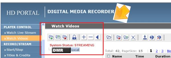
To stop the recording and create an archived file, press the Stop button to begin the “indexing” process. Depending on the length of the archived material, this could take a few seconds up to several minutes to complete.
