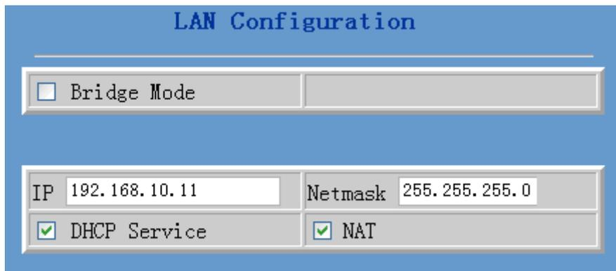
The screenshot shows a blue-tinted window titled "LAN Configuration". At the top, there is a checkbox labeled "Bridge Mode" which is currently unchecked. Below this, there are two input fields: "IP" with the value "192.168.10.11" and "Netmask" with the value "255.255.255.0". At the bottom, there are two checkboxes: "DHCP Service" and "NAT", both of which are checked.
