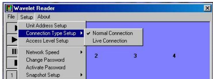
To establish a Live Connection, select **Setup → Connection Type Setup → Live Connection** from the menu bar.
