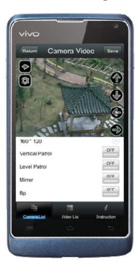
C.» (Via mobile Broswer to view the camera: Open your mobile broswer, then input the DDNS address(xxx.vipcam.org) or ip address of the camera.
