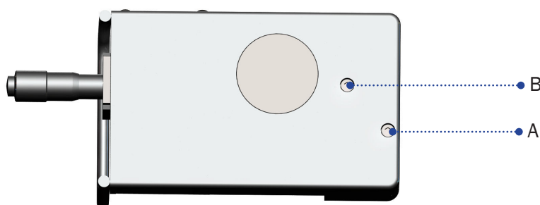
Figure 4.6 The two screws holding the transducer house in place
