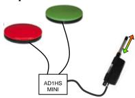
AD1HSMINI is a driver for control of an actuator/motor so that it can be controlled independently of the electronics of the chair. It is a separated unit and is as such not dependent on the type of chair it is mounted on. For the same reason it is necessary to turn the chair on to activate the actuator through AD1HSMINI.
