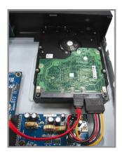
Step4: Align the screw hole on the each bracket with the screw hole on the each side of the HDD as shown below, and fix the HDD to the bracket with a HDD screw supplied.
