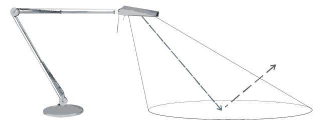
For right handed users, the luminaire should be positioned on the left side to prevent shadows in the work-field. For left-handed users, the correct position is right side.
