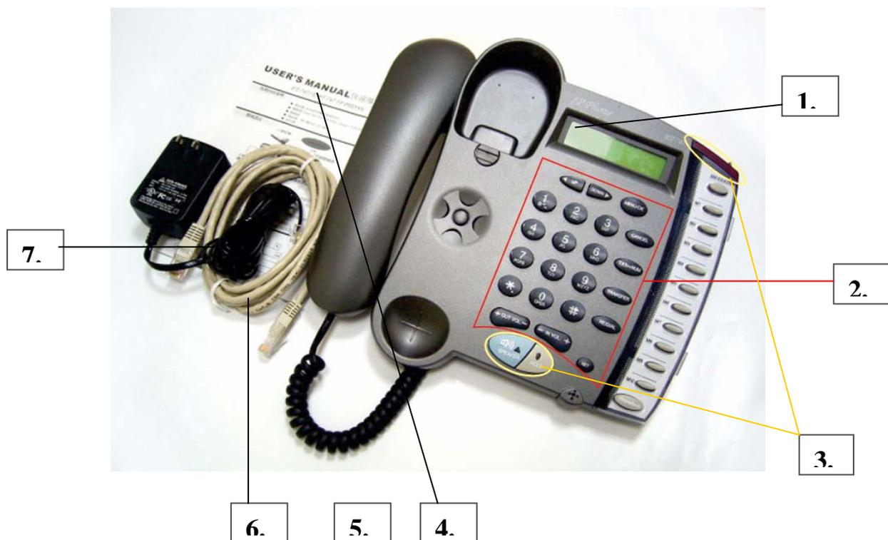
Figure 1. Key parts of the IP0120/IP0121 IP Phone
