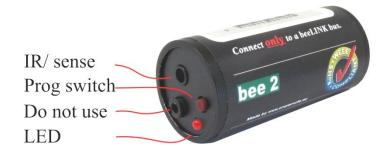
The IR/ sense socket is output for the IR-emitter that sends IR to the device to be operated. In some cases this socket is also used for sensing purposes. Some BeeLINK2 converters needs to know if the device is powered up or not.
