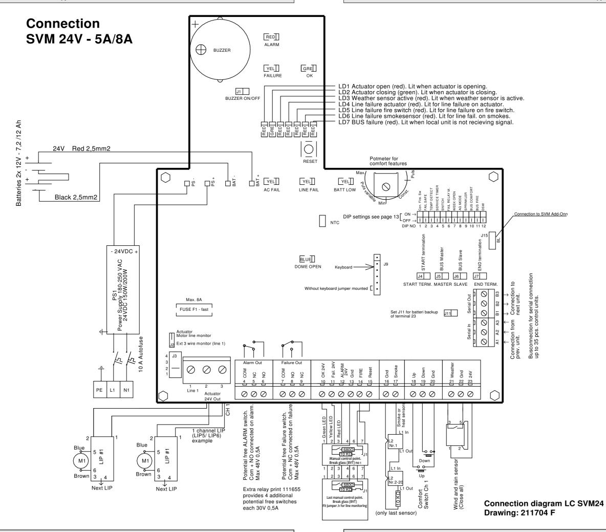
Control for Fire and Comfort Ventilation Type SVM 24V-5A / SVM 24V-8A
