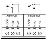
Extra relay print 111655 provides 4 additional potential free switches each 30V 0,5A
