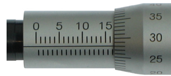
Figure 5.7. Example 2: Reading = 16.78mm
