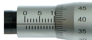
Figure 5.6 Example 1: Reading = 10.38mm
