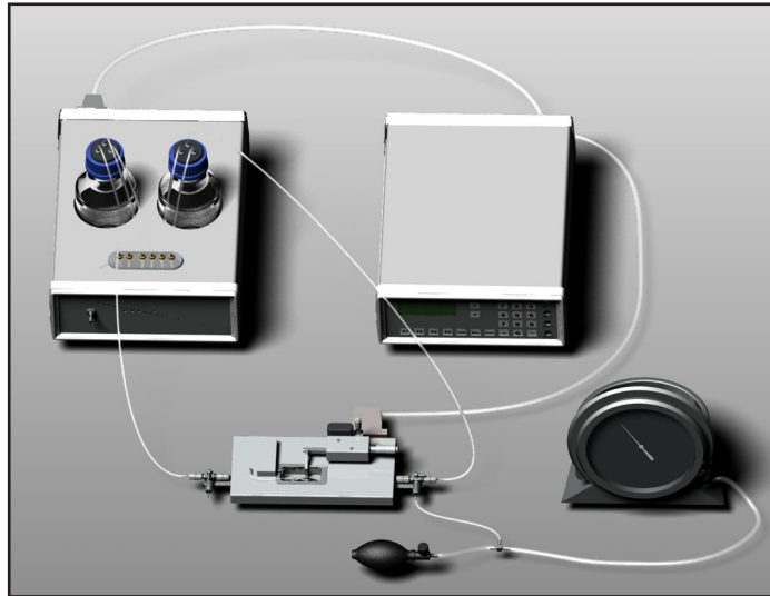
Figure 5.11 Illustration of set up for pressure transducer calibration
