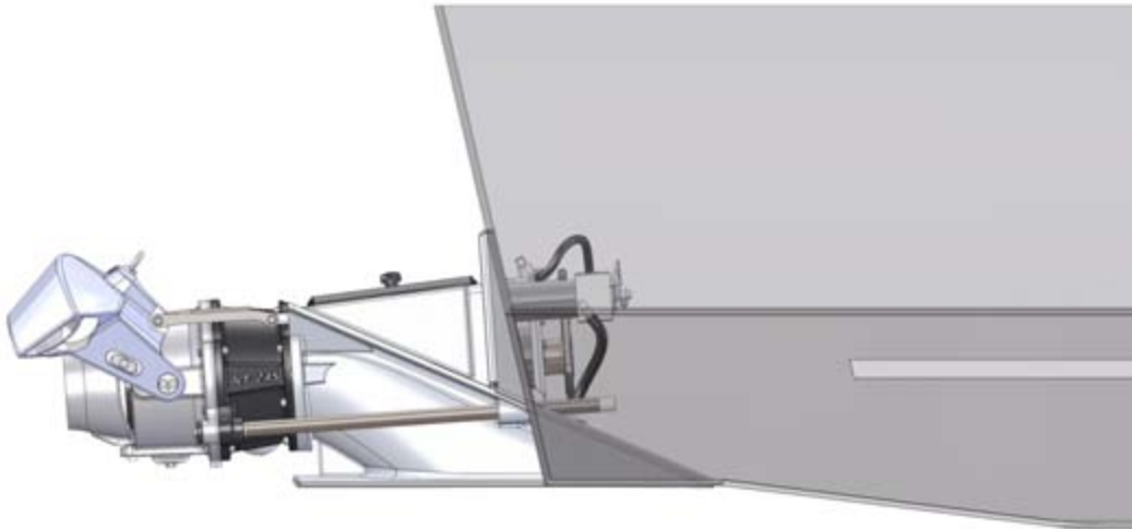
Figure 2. Long tail installation
