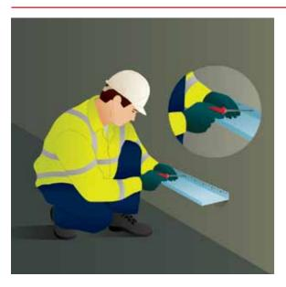
Starter tracks should be fixed prior to installing the insulation boards. Starter tracks must not be fitted below the DPC line and must be a minimum of 150mm above ground level (unless specified otherwise). Starter tracks are to be fitted using ROCKWOOL Base Profile Fixing Screws at maximum 300mm centres. Packers should be used on uneven substrates. Adjoining lengths must be connected using ROCKWOOL Base Profile Connection Clips and levelled using a spirit level.
