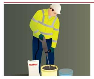
Weather conditions must be closely monitored during the application of the dashing mortar. ROCKWOOL Brick Effect Base Coat should be properly prepared by thoroughly mixing a full bag of the specified base coat with 4.4 to 5 litres of clean, cool water using a slow rotation drill with a suitable mixer. After achieving a homogenous mix, free from lumps, leave for 5 minutes and then mix again. Once prepared it should be used within 1 hour, mixing every 30 minutes.
