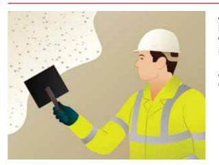
Apply the aggregate to the ROCKWOOL Dash Receiver using a hawking trowel to the agreed coverage. For best results, flick the wrist with the trowel parallel to the render at the time the aggregate is released.
