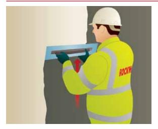
Weather conditions must be closely monitored during the application of the base coat. The temperature must not be below 5°C on a falling thermometer or below 3°C on a rising thermometer (ensuring it rises above 5°C). There must be no risk of frost within 48 hours of application.
