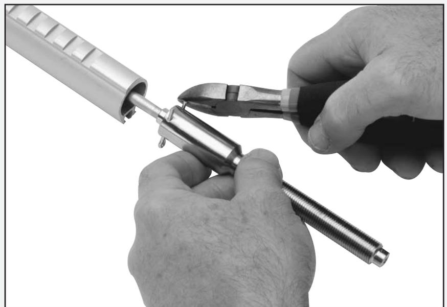
Assemble turnbuckle and attach Harken toggle.
