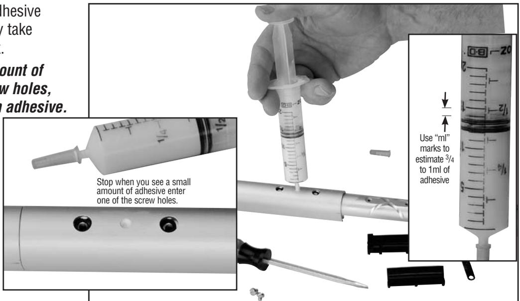
Tighten screws into connector holes. Make sure a drop of adhesive entered each screw hole. If not, apply to screw.
