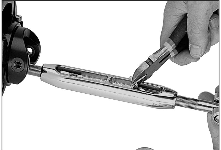
Slide lower drum assembly over turnbuckle and attach using long crosspin. Use plastic washers provided.
