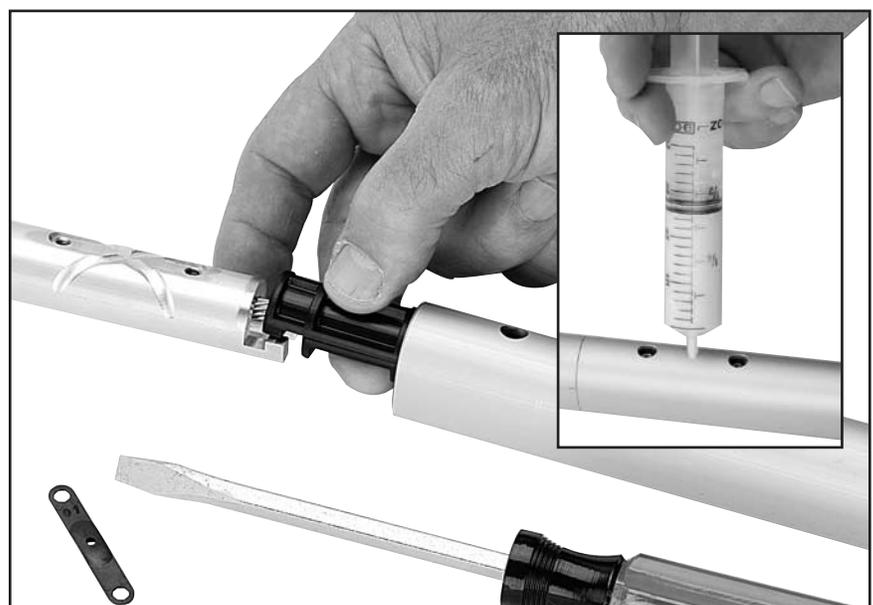
Continue installing connectors and wedges. Make sure to use adhesive in screw holes.
