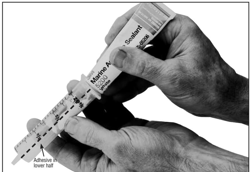
Start plunger into injector and immediately hold upright so plunger is down and applicator tip is up.
