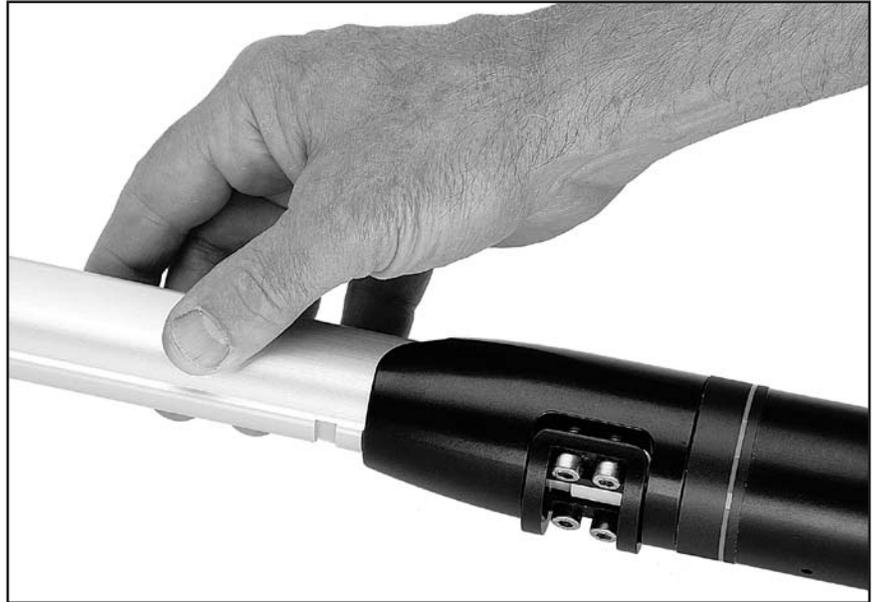
Slide halyard swivel above feeder. Place feeder in foil recess. Push screw down so tab catches under foil. Tighten screw.
