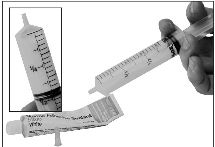
Put a drop of adhesive into screw holes.
