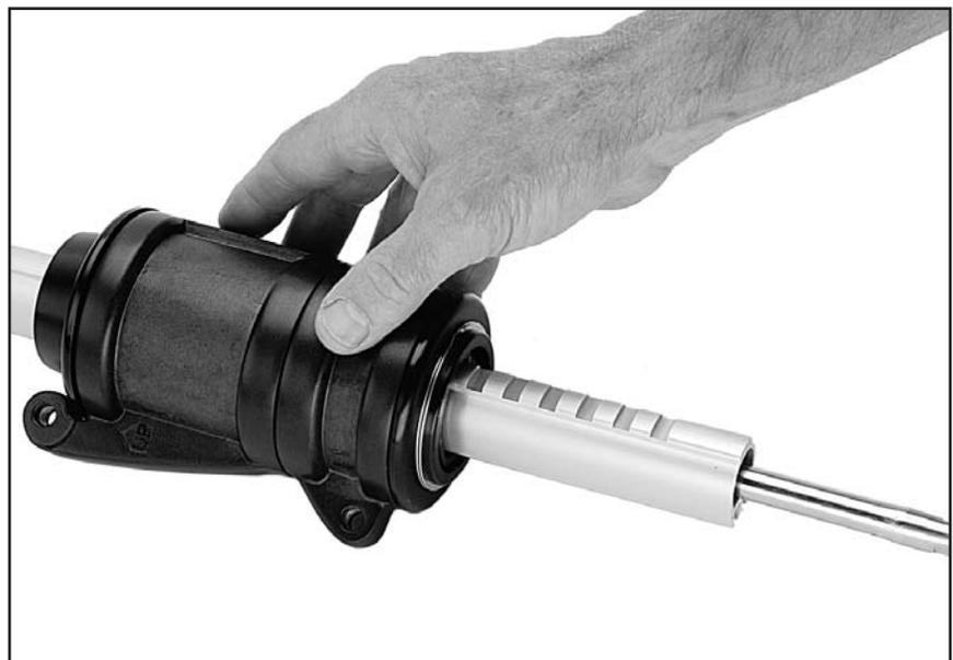
Loosen foil clamp screws at top of drum assembly.
