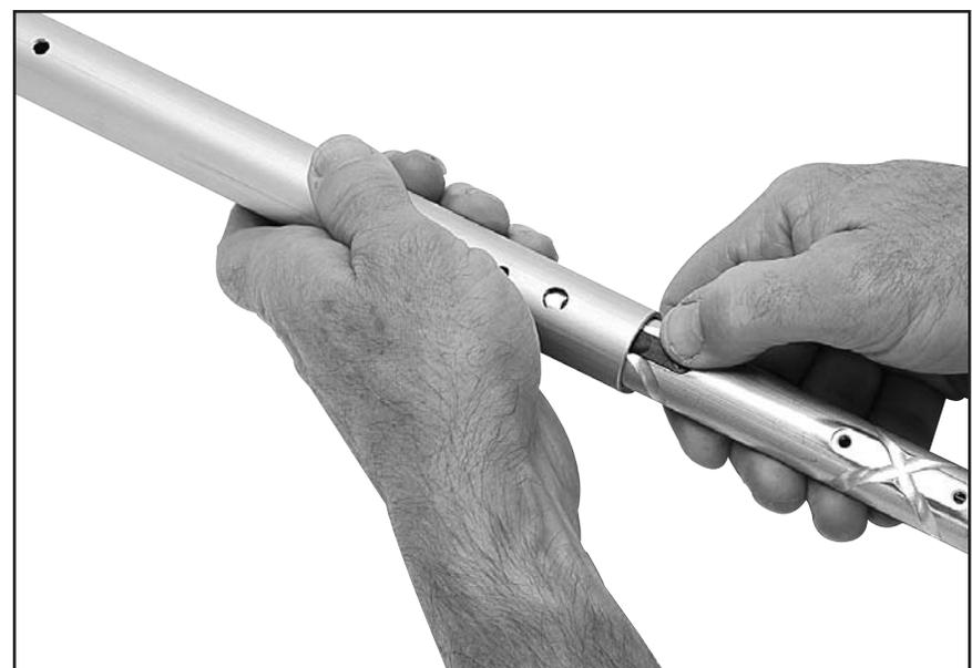
Inject only a small amount of adhesive into middle hole. Unit 2 will only take 3/4 to 1ml of a graduation mark.
