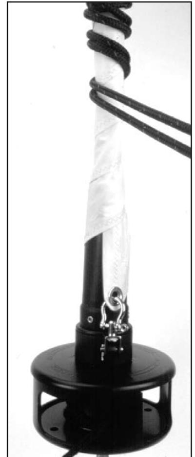
Race conversion allows use of both grooves for sail changes and tacking genoas on deck for use of maximum luff length genoas.
