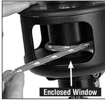
Run line through enclosed window in guard and into hole in bottom plate of spool. Tie a small overhand knot and pull it up under drum assembly.
