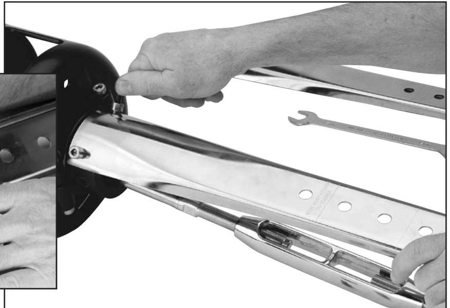
Fasten second long link plate to drum assembly and secure to clevis pin using locknuts.
