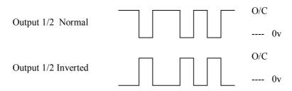
Using the internal open collector transistor max sink current is 100mA.
